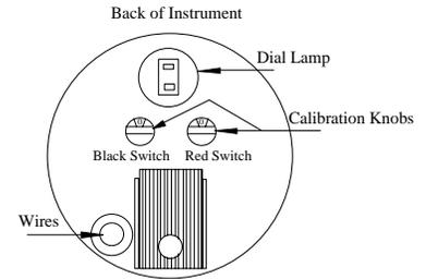
There are two calibration switches on the back of the instrument, Black and Red. Both are required for calibration. If there's an existing tachometer, or you know the engines' idle RPM, you can calibrate the tachometer without referring to Tables I, II, or III.
