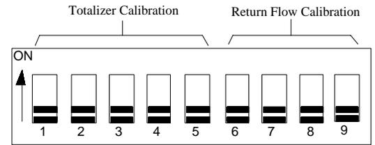
There are nine, “Dip” switches located on the back of your 6500 Series Instrument. These switches are used to calibrate the instrument prior to use. Switches 1 through 9 are shipped in the OFF position.
