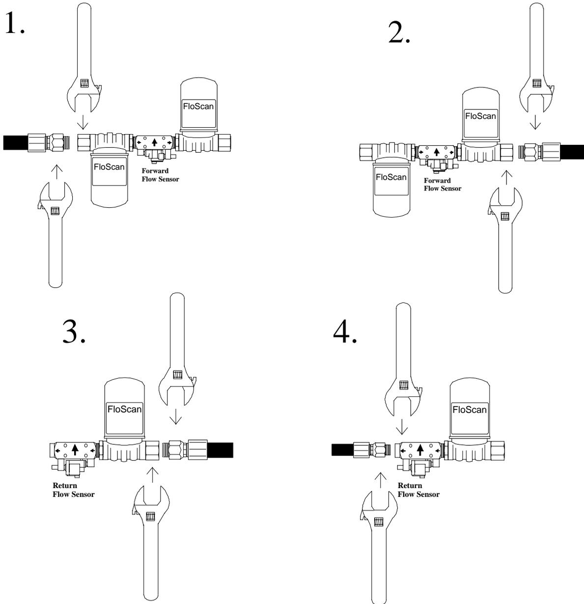
Always assemble hose ends and fittings into sensor assemblies using two wrenches, (at places indicated in the drawings). One wrench is used to turn the hose end or fitting into the sensor assembly, The second acts as a back-up or counter torque wrench and is applied to either the steel SAE/Female pipe adapter fitting, or the Return Sensor's aluminum block at its outlet port.
