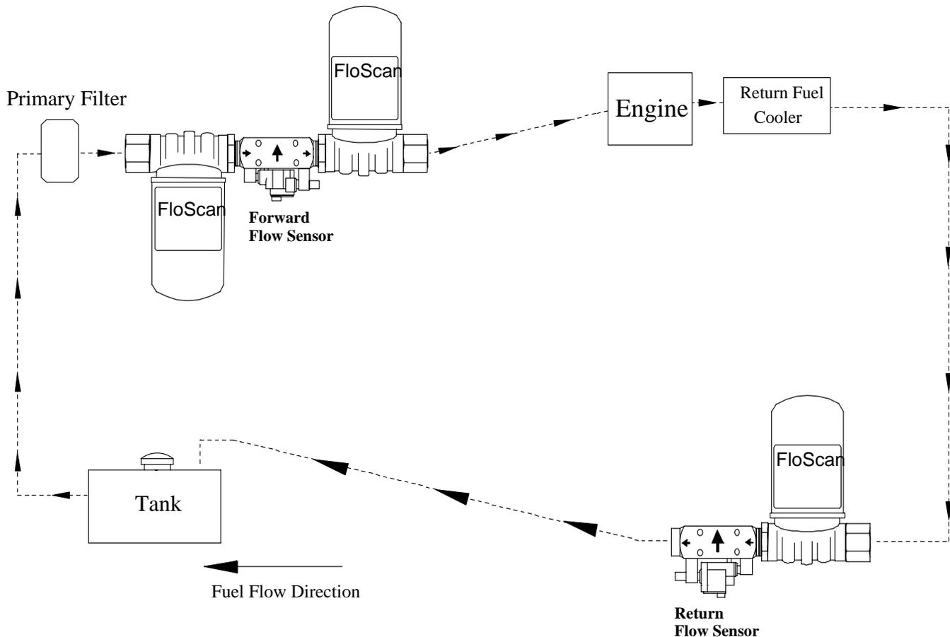
**\*Caution: Diesel System Components are not designed for use on Gasoline Fuel Systems.**
