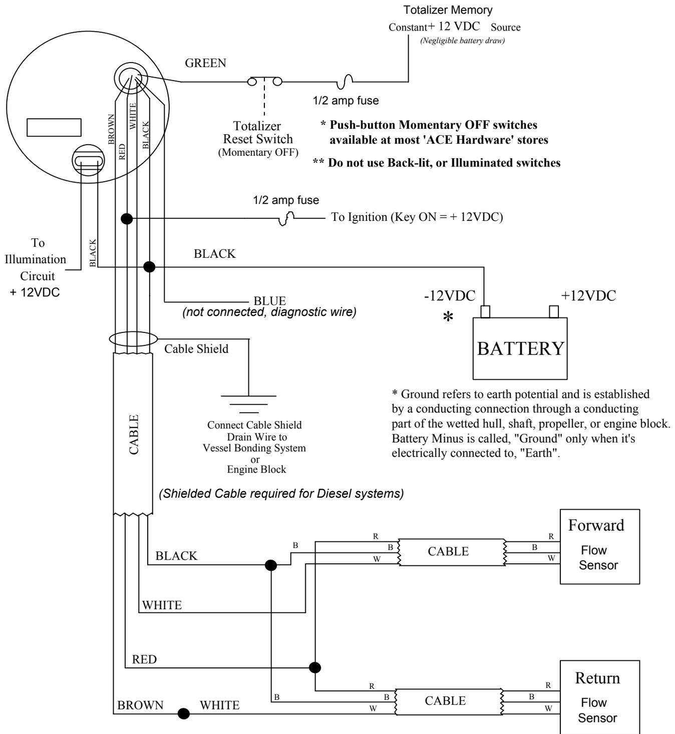
**NOTE:** For twin engine installations, you will repeat the wiring shown above for each engine.
